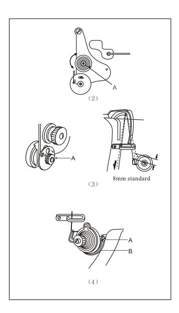
2. Adjusting the tension of needle thread
